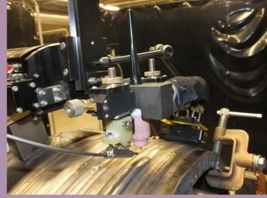
ealed system at repair location in-reactor (mock-up trials shown – ECA for first inspection,
