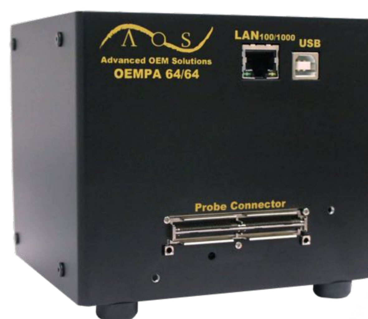
64-elements-PA instrument from AOS NDT with fast acquisition (150 MB/s)
